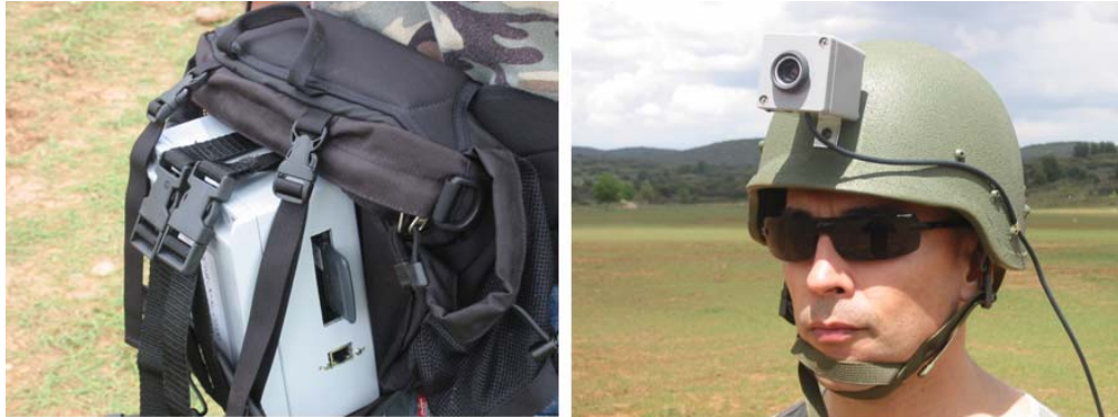
SBC with WiFi card and video camera mounted on helmet
